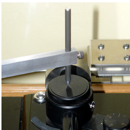
Figure 3 – Close-up of Nerve Audio Cartridge Alignment Protractor showing Pivot Pointer centered on top of tonearm bearing assembly.
